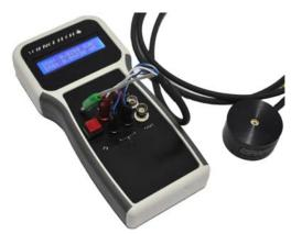
SOL-METER-D Digital Power Meter With Reference Detector
