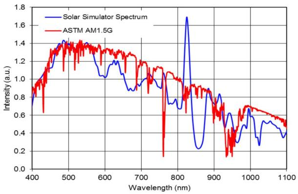
Solar simulator spectrum compared with ASTM AMI.5G solar spectrum
